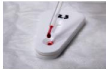
4. Add 2 drops (approx. 60µl) of specimen to the sample port in the device.
